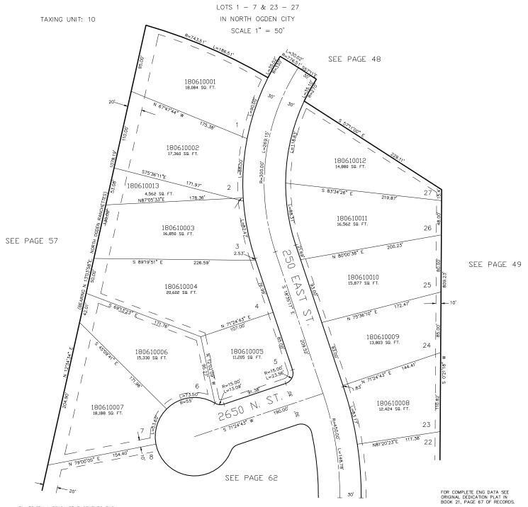
7' UTILITY & DRAINAGE EASEMENTS EACH SIDE DF PROPERTY LINES AS INDICATED BY DASHED LINES EXCEPT AS OTHERWISE SHOWN.
